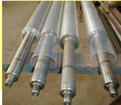
Sleeves installation on aluminium rolls
