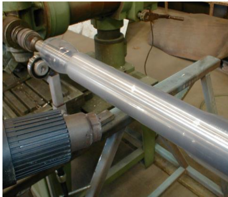
Sleeves installation on aluminium rolls
